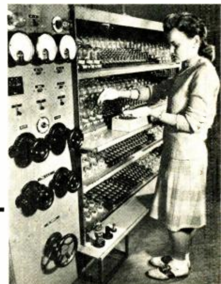
RCA special aging rack for miniature tubes.
